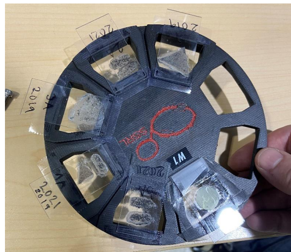
Applying thin section soil samples for \mu -XRF and \mu -XAS experiments at the 2-3 beam line at Stanford Synchrotron Radiation Lightsource.
